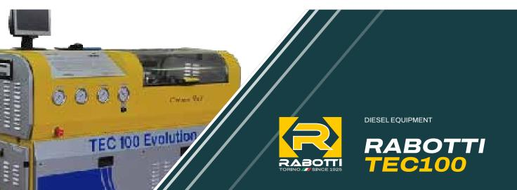
TEC100 Test Bench is a versatile and high-performance diagnostic tool designed for comprehensive testing of common rail injectors and pumps across multiple brands, including Bosch, VDO/Continental, Delphi and Denso. It operates as an independent unit, eliminating the need for external dependencies while ensuring precise and reliable results.
